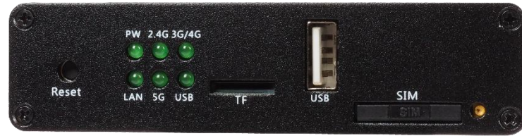
Reset button LEDs SD card slot USB port SIM slot SIM release button
